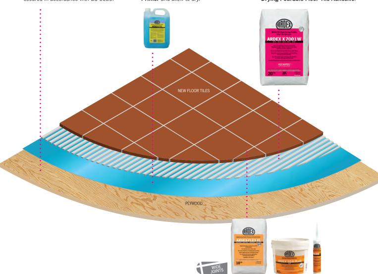
4. Grout the joints using **ARDEX-FLEX FL Flexible Tile Grout**.
